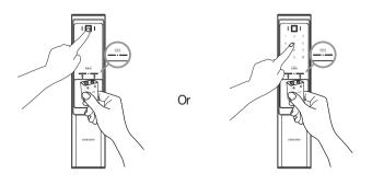
While connecting a 9V battery to the external power (emergency battery) contact point, recognize a fingerprint or press a master/user password.
