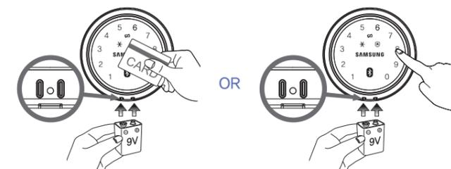
While contacting a 9V battery to the external power (emergency battery) contact on the outer body for 2 seconds or longer, place the card or key tag or enter the password.
