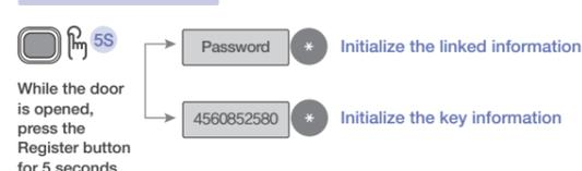
While the door is opened, press the Register button for 5 seconds
